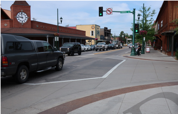
Bulbouts with gentler turning radii and roll-up curbs in Downtown Whitefish, MT.
